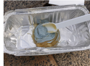
❸ Mix the pigment into the glue – add small amounts of pigment and mix to ascertain the overall colour and whether more is needed
